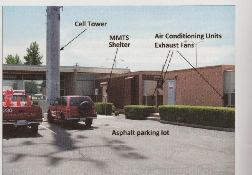
Figure 5. Temperature station at the Marysville, California fire department surrounded by heat sources.
